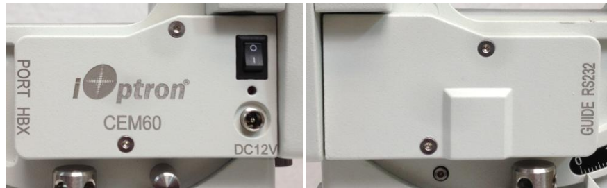
Figure 2. Ports on a CEM60 mount
